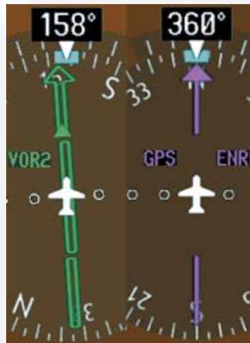
Figure 609-5: Course Deviation Indicator (VOR and GPS)
