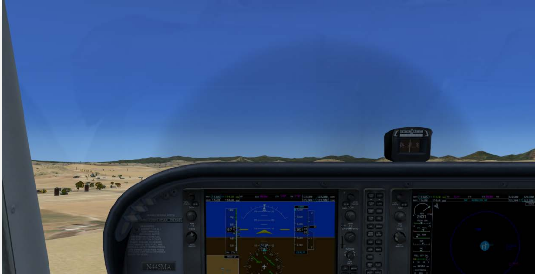
Figure 304-10: V_y Pitch Attitude
