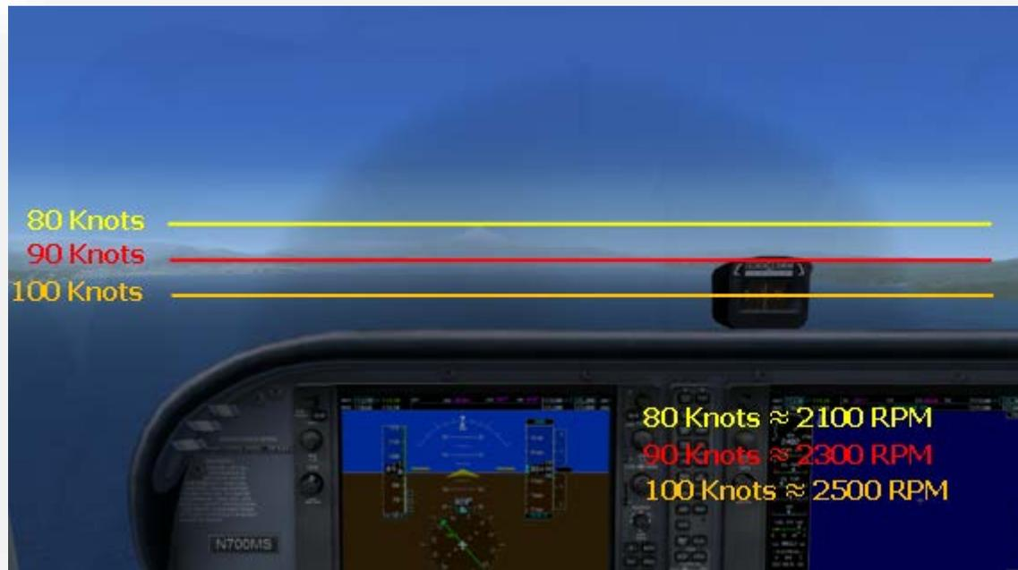
**Figure 101-3:** Pitch and Power Settings for Level Flight
