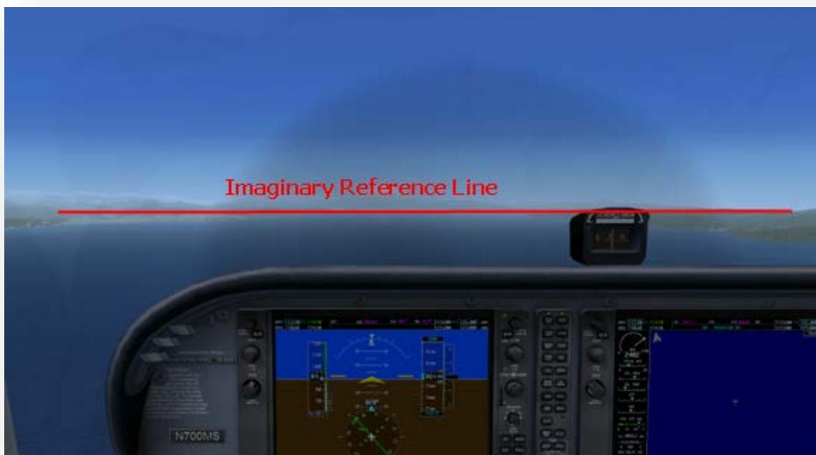
**Figure 101-2:** Level Flight at 90 Knots
